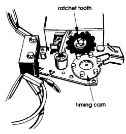
**3.** Turn the timing cam by hand until the "V"-shaped notch lines up below the ratchet tooth.
